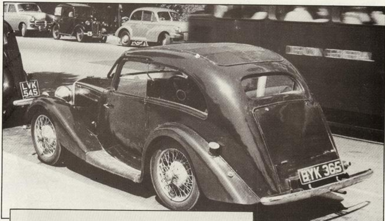
1935 Cresta saloon, photographed at Poole, in Dorset, during the Fifties, clearly shows the pillarless construction.
