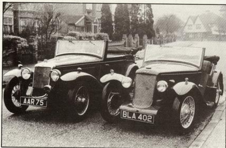
Hillman variant of the March two seater, photographed ca. 1956 probably at Brands Hatch. Note the lack of louvres in the top of the bonnet.
